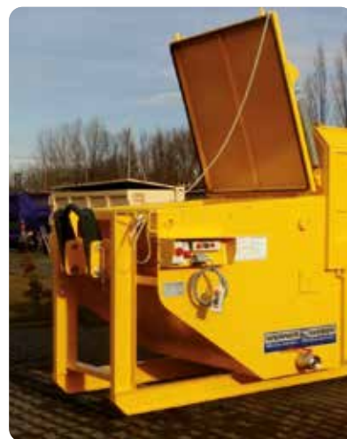
Cover over filling opening
